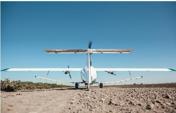
The face of agriculture is changing with aerial drones that will replace the traditional crop duster, with speed, efficiency, and cost benefits, capable of spraying up to 135 acres an hour with one half the cost of traditional spraying, especially valuable for vineyards, which can be dangerous for tractors. Watch the skies for **Pyka** (Silicon Valley) and **Volocopter** (Germany) to take to the skies for autonomous aerial sprayers. (*Progressive Farmer, August, 2020*).
